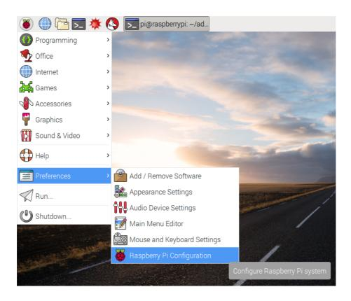
Ensure the camera software is enabled:
